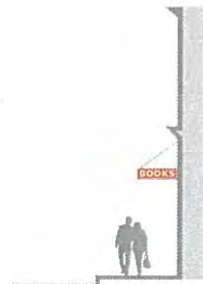
Canopy Fascia Sign
